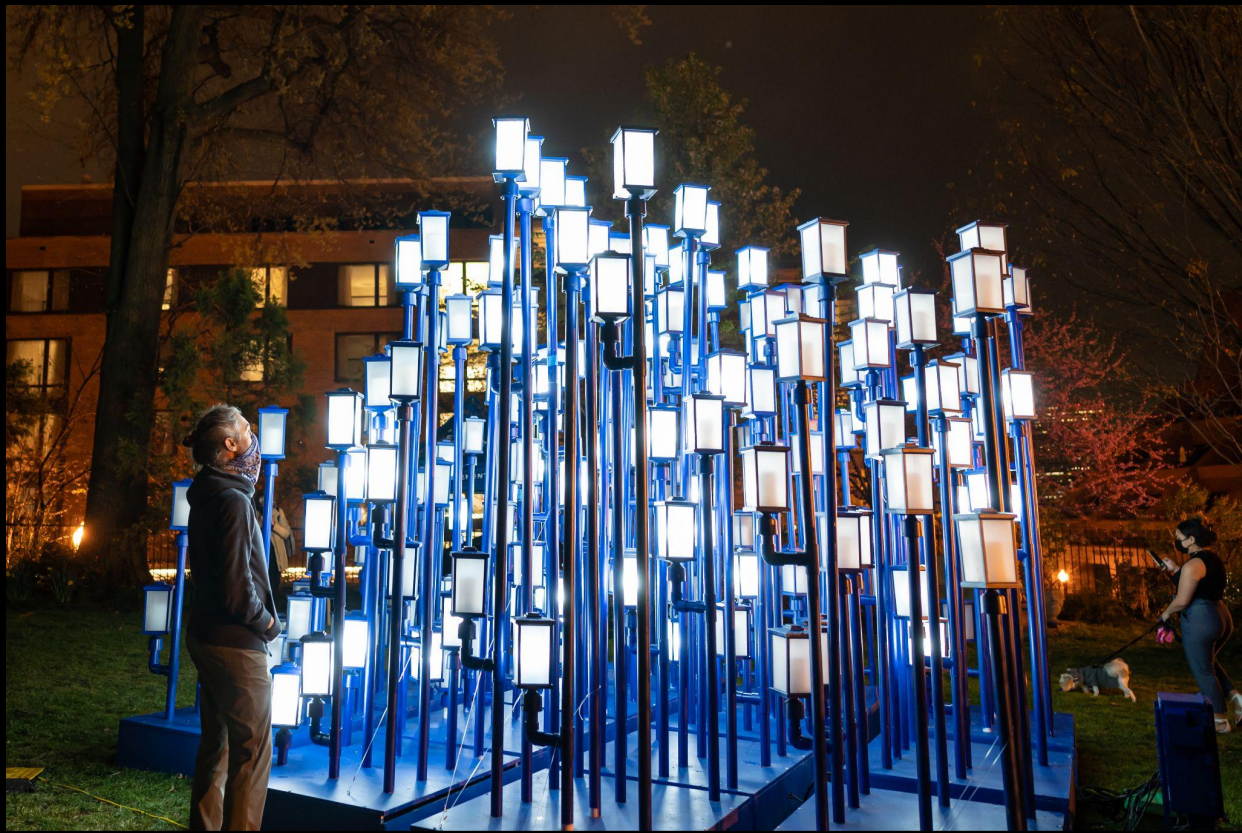
“Madness Method” (with David Greenfieldboyce). 216 computer-controlled lanterns outside for three months. PCA9685, diff-i2c, Pi 4, three hot controllers w/ arbitration by AVR hardware watchdog
